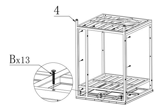
STEP 6 Attached the Right side panel (3) with 11 pcs of M6\*40 screws(B).
