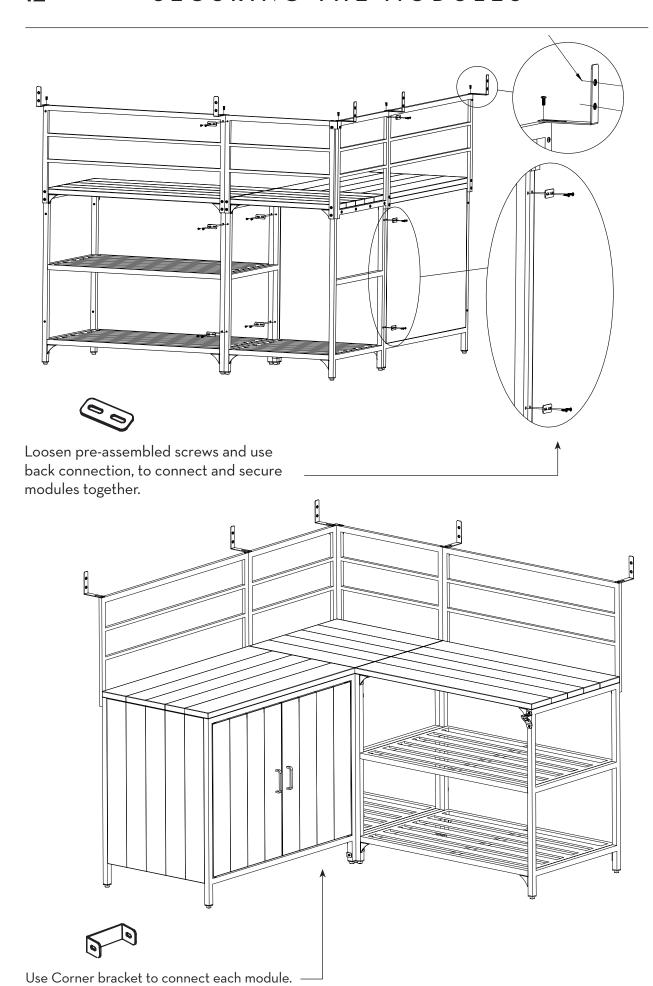
Use Wall connection to secure each module to prevent the modules from overturning.
