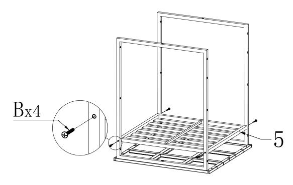
STEP 4 Attach the bottom panel (6) on the frame with 2 pcs of M6\*40 screws(B).
