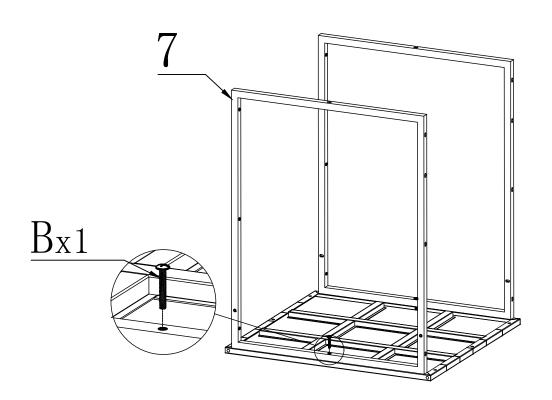
STEP 3 Attach the shelf (5) to the front- and back frame (7, 8) with 4 pcs of M6\*40 screws(B).
