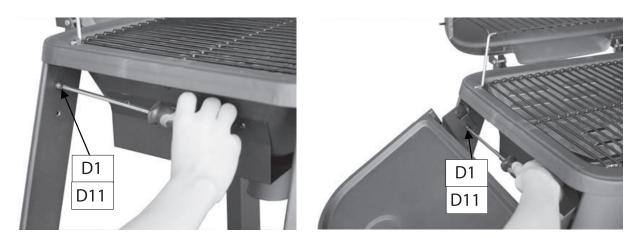
**19.** Slide a Shelf Spacer (DII) onto a M6x15 Bolt (DI) and screw it into the upper fixing point on the left rear leg as shown. Repeat for the left front leg. Attach the previously assembled Side Shelf (CI) to the left hand side of the barbecue by sliding a Shelf Spacer (DII) onto a M6x15 Bolt (DI) and fitting the shelf to the lower fixing point on the rear leg as shown. Repeat for the front leg.
