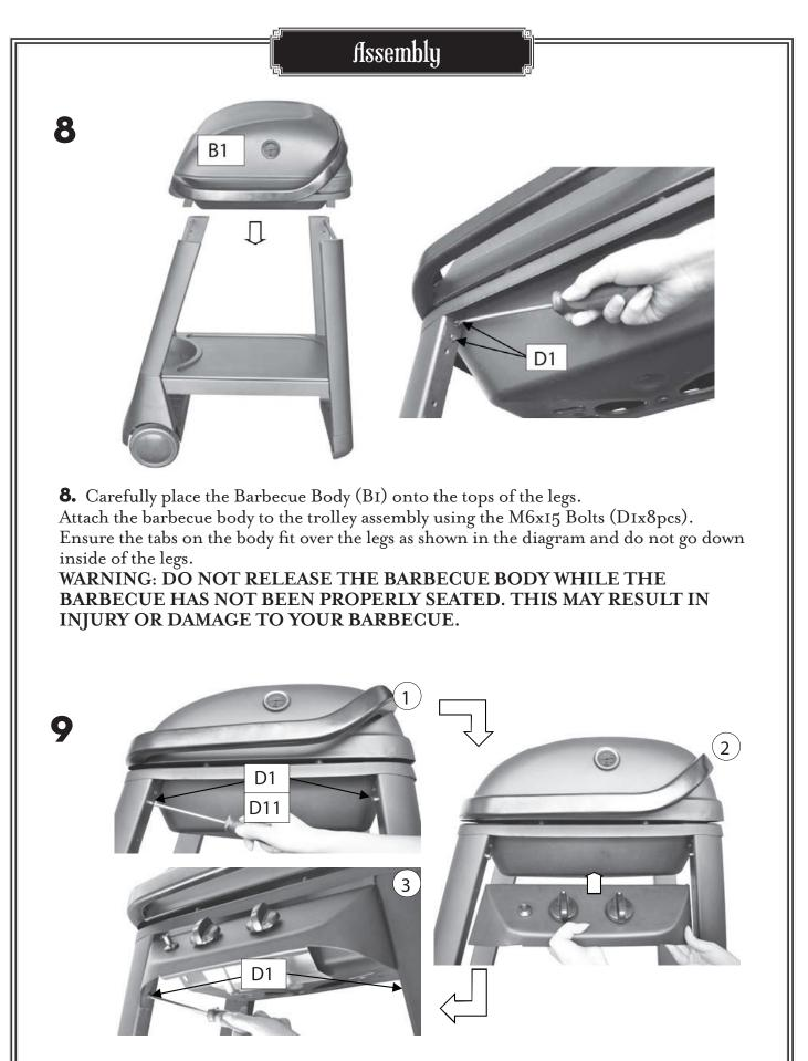
**9.** Install a M6x15 Bolt (D1) and a Spacer (D11) into the upper fixing hole on each front leg. Place the Control Panel (B3) assembly in position by aligning the spacers with the slot on each side of control panel and fix it onto the trolley assembly using M6x15 Bolts (D1x2pcs).
