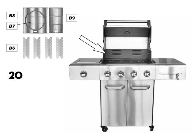
**20.** Lay the Flame Tamer (B6) carefully into the body ensuring it lies level within the body. Lay the Left Cooking Grill (B8) and Right Cooking Grill (B9) and Round Grill (B7) into place.
