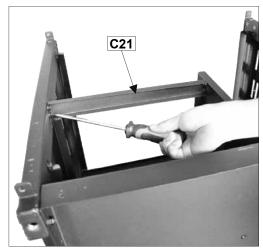
**5.** Attach the Food Basket Front Bracket (C21) to the Left Cabinet Panel Assembly (C9) and Middle Panel (C18) using M6x15 Bolts (D2x4pcs).
