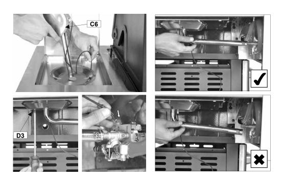
**16.** Feed the venturi tube of the Side Burner (C6) through the hole in bottom of the side burner shelf, and fix side it onto side burner shelf using a M4xIO Bolt (D3) as shown.
