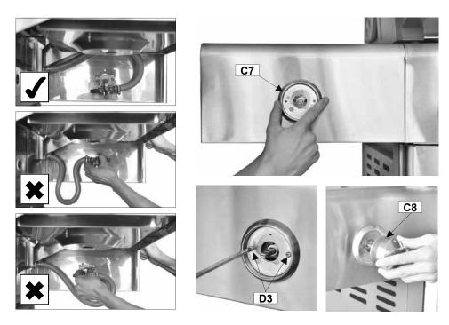
**15.** Attach the side burner valve and Knob Bezel (C7) onto side burner shelf using M4xIO Bolts (D3x2pcs) as shown. Press the Side Burner Knob (C8) onto side burner valve stem.
