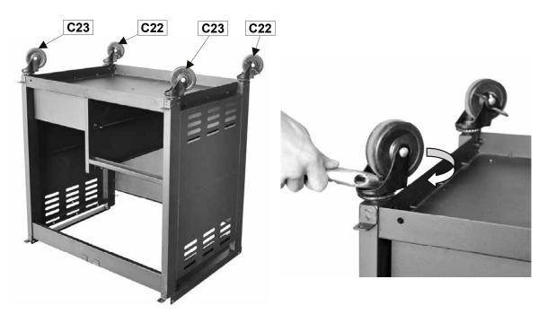
**7.** Carefully turn the cabinet upside-down. Attach the Lockable Casters (C22x2pcs) into the rear side holes of the left/right cabinet panel assembly and the Casters (C23x2pcs) into the front side holes of the left/right cabinet panel assembly.
