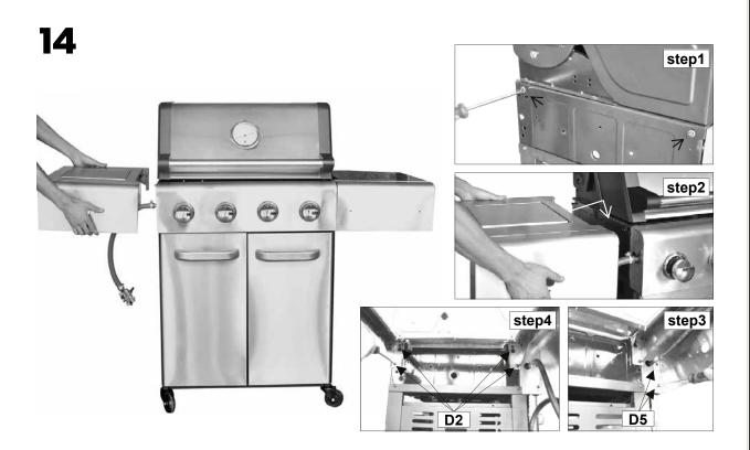
**14.** Attach the side burner shelf assembly to the barbecue body using ST4.0xIO Screw (D5x2pcs) and M6xI5 Bolts (D2x4pcs) as shown.
